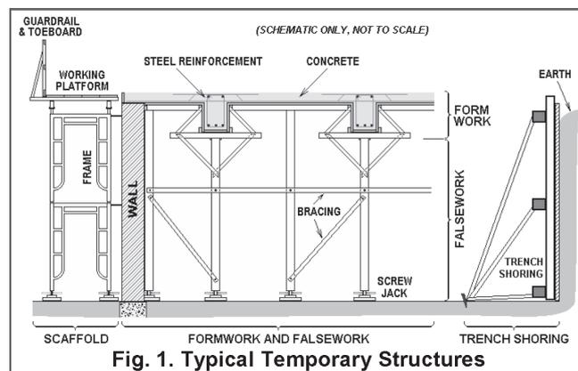
Fig. 1. Typical Temporary Structures
