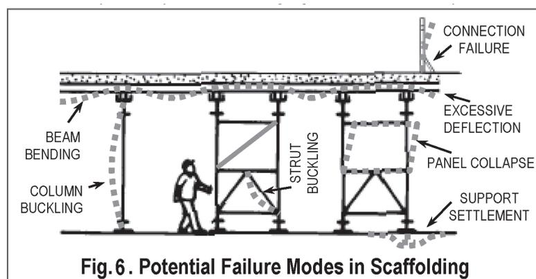
**Fig. 6. Potential Failure Modes in Scaffolding**
