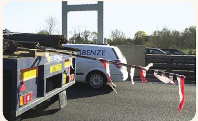
Figure 9: Rebar transportation hazard.
